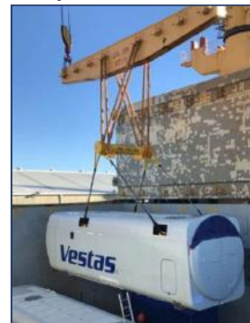
Unloading of Wind Turbine Nacelles at Geelong First Shipment of 15 Nacelles
